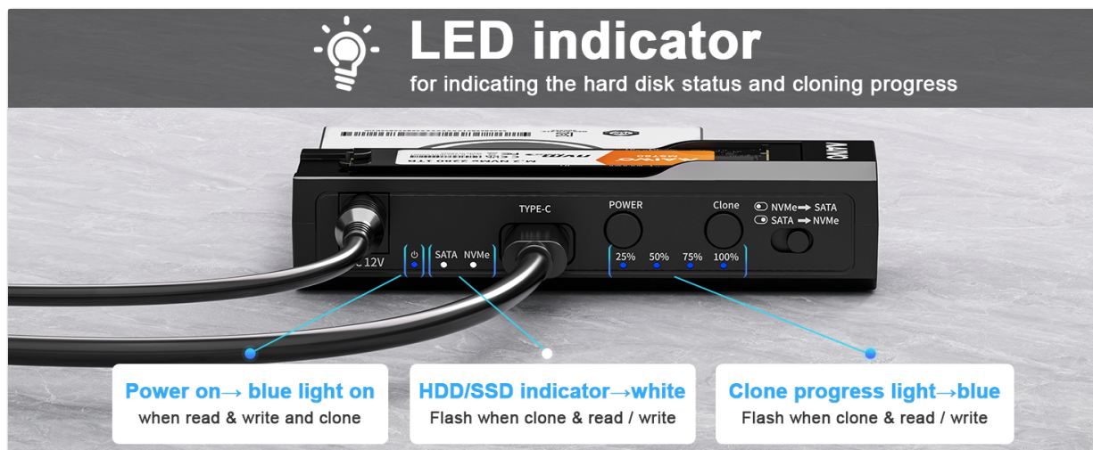
Image 6.3: Understanding the LED indicators for device status and cloning progress. For a visual demonstration of the offline cloning process, please watch the video below:
