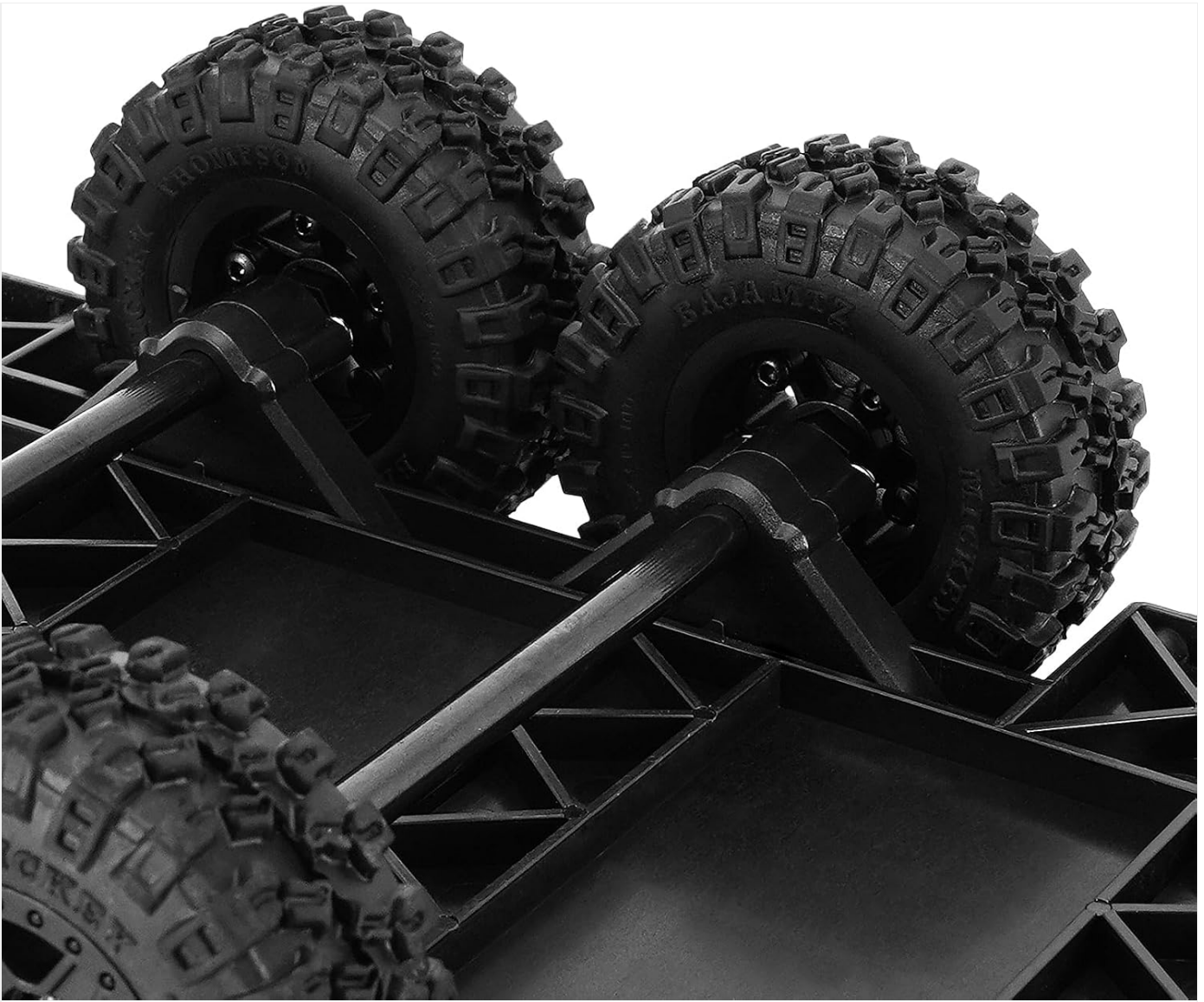
Image: Underside view of the trailer, highlighting the dual axle design for stability and load distribution.
