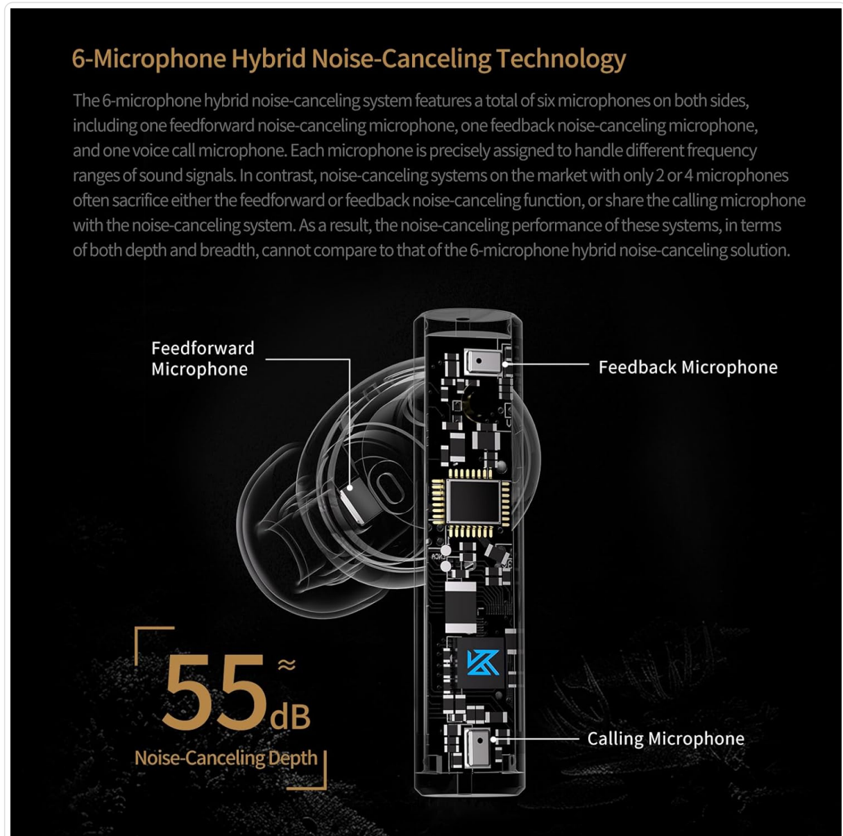
Figure 2: Illustration of the 6-microphone hybrid noise-canceling system.
