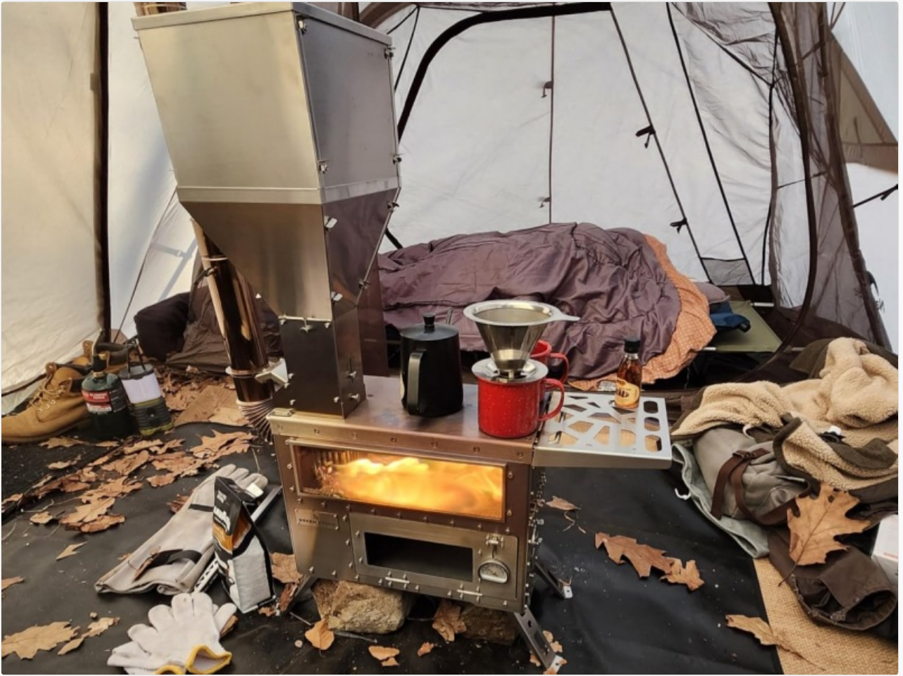
Image 4.3: The pellet hopper attached to the stove, ready to feed pellets into the combustion chamber.
