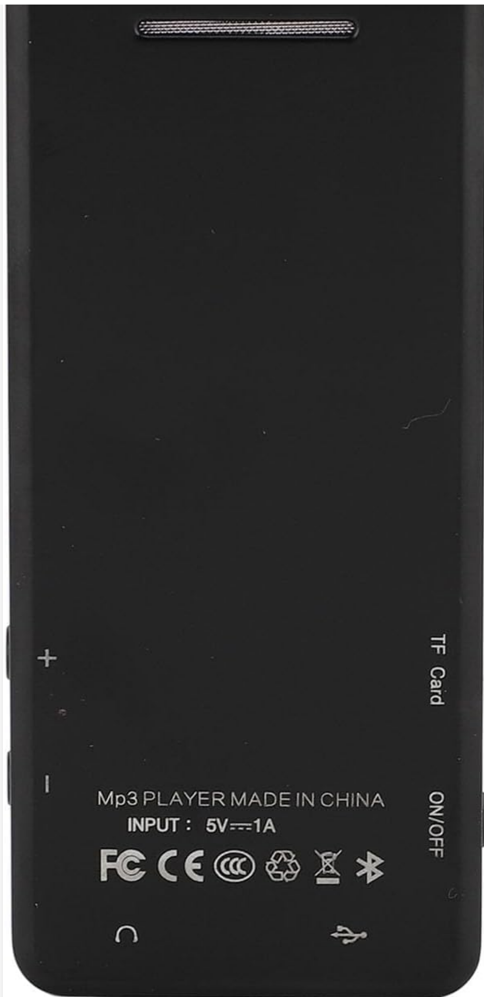
Image: Back view of the Pomya MP3 Player, highlighting the TF card slot for expandable storage, the 3.5mm headphone jack, and the USB charging port. Device information and regulatory marks are also visible.
