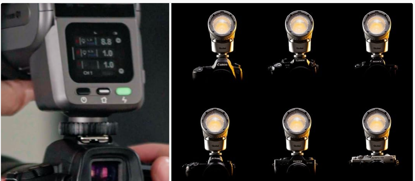
Image 6.3: The HS Freeze Q1 display showing adjustable color temperature and brightness settings for the continuous LED light.
