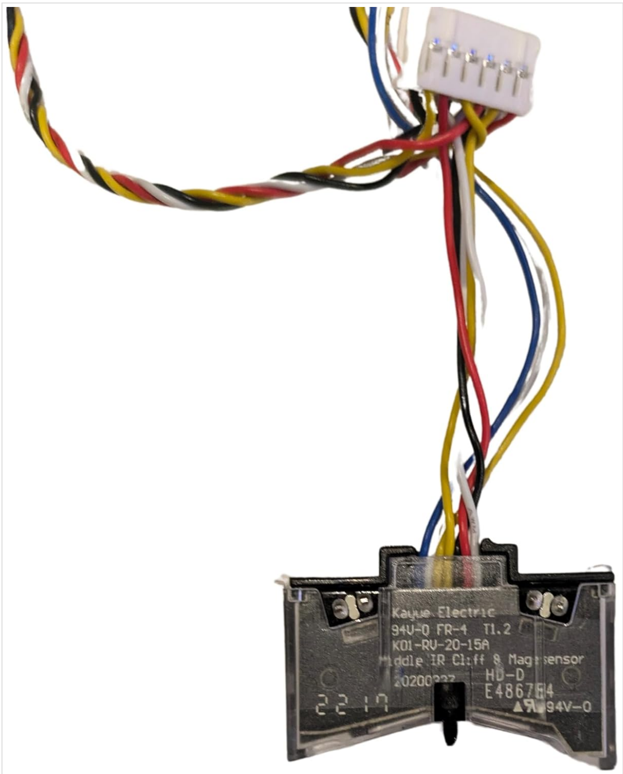
Image 2: Detailed view of one cliff sensor, highlighting the wiring and connector.
