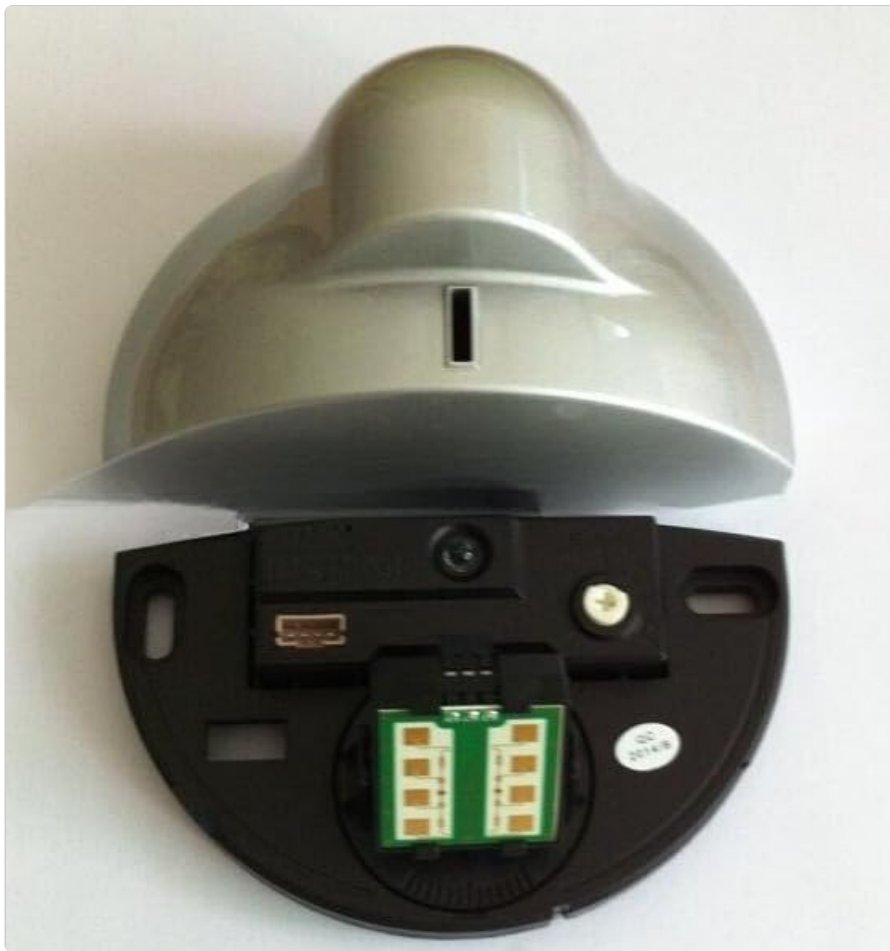
Figure 1: yancinne ATF830 Automatic Door Sensor Probe (Half Circle Style). The image displays the sensor's silver outer casing detached from its black base, revealing the internal circuit board with gold contacts.
