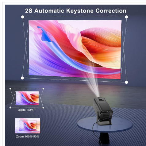
Figure 5.3: Automatic keystone correction ensures a perfectly rectangular image.
