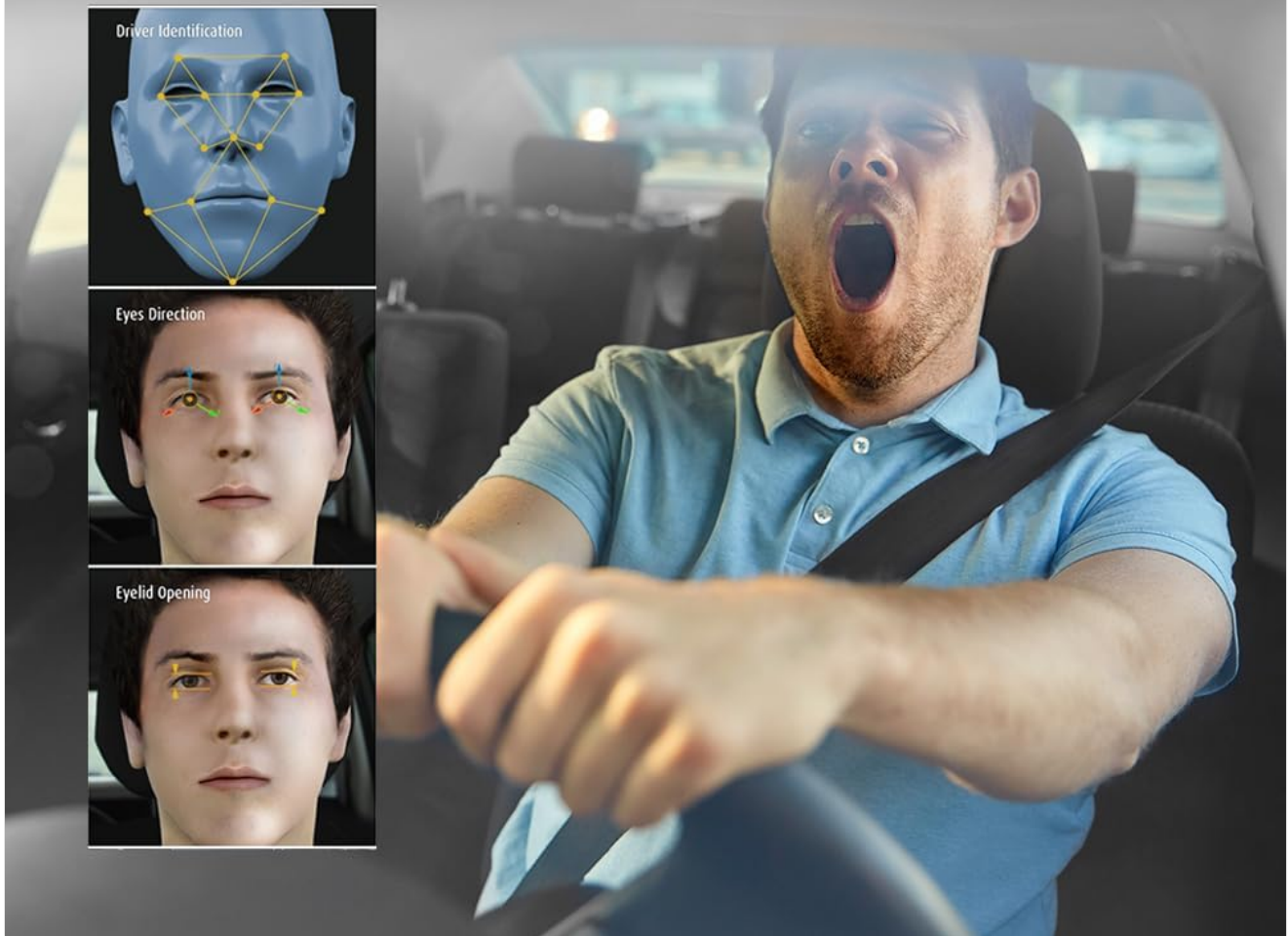
Figure 4.3: Visual representation of Driver Fatigue/Distracted Monitoring (DMS) capabilities.
