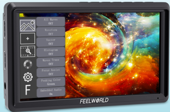
Image: Intuitive controls and menu interface of the FEELWORLD FW568 V2 monitor.
