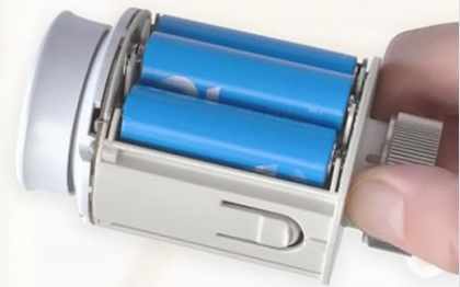
Figure 4.1: Tool-free installation process and battery compartment for the EZAloT thermostat.
