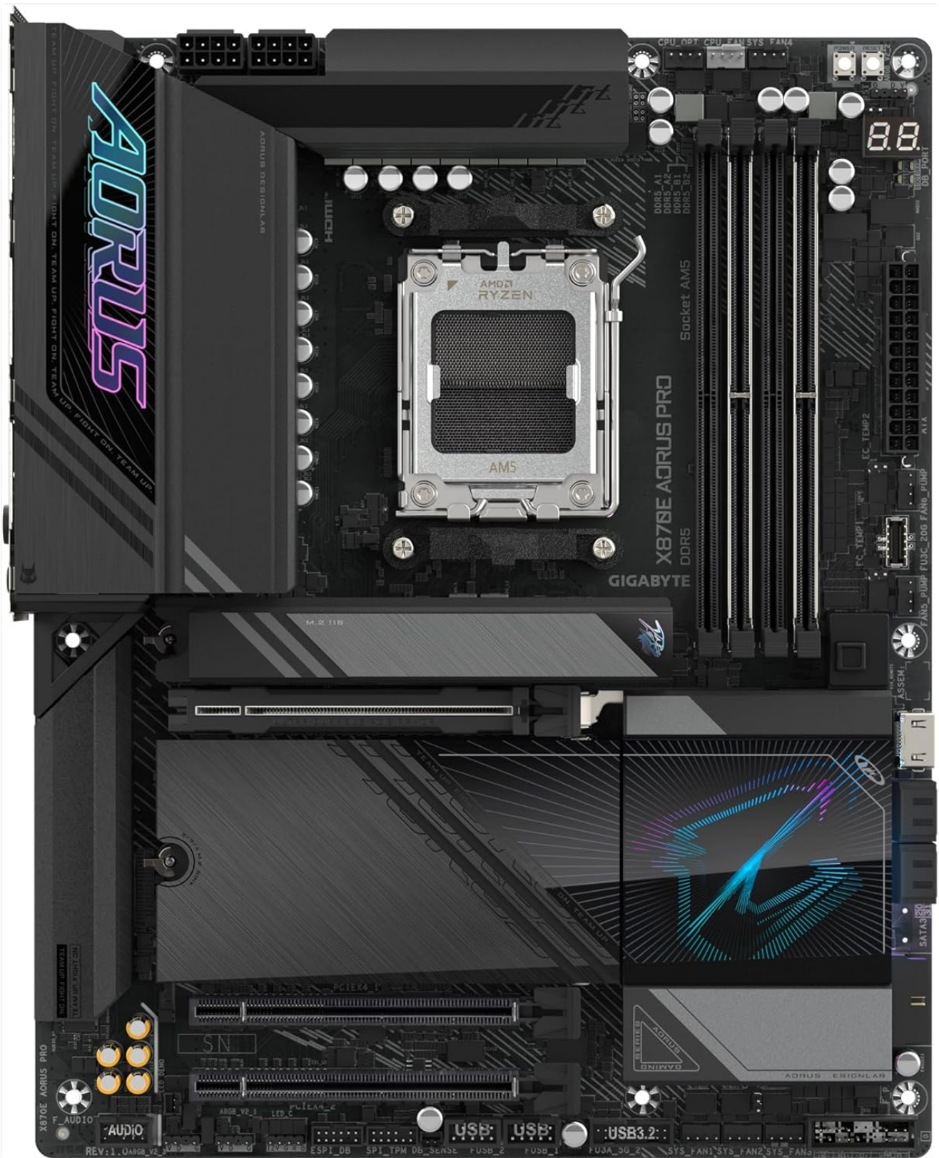
Figure 2: Top-down view of the GIGABYTE X870E AORUS PRO Motherboard. This image provides a clear overhead perspective, showing the CPU socket, DIMM slots, PCIe slots, and various headers.
