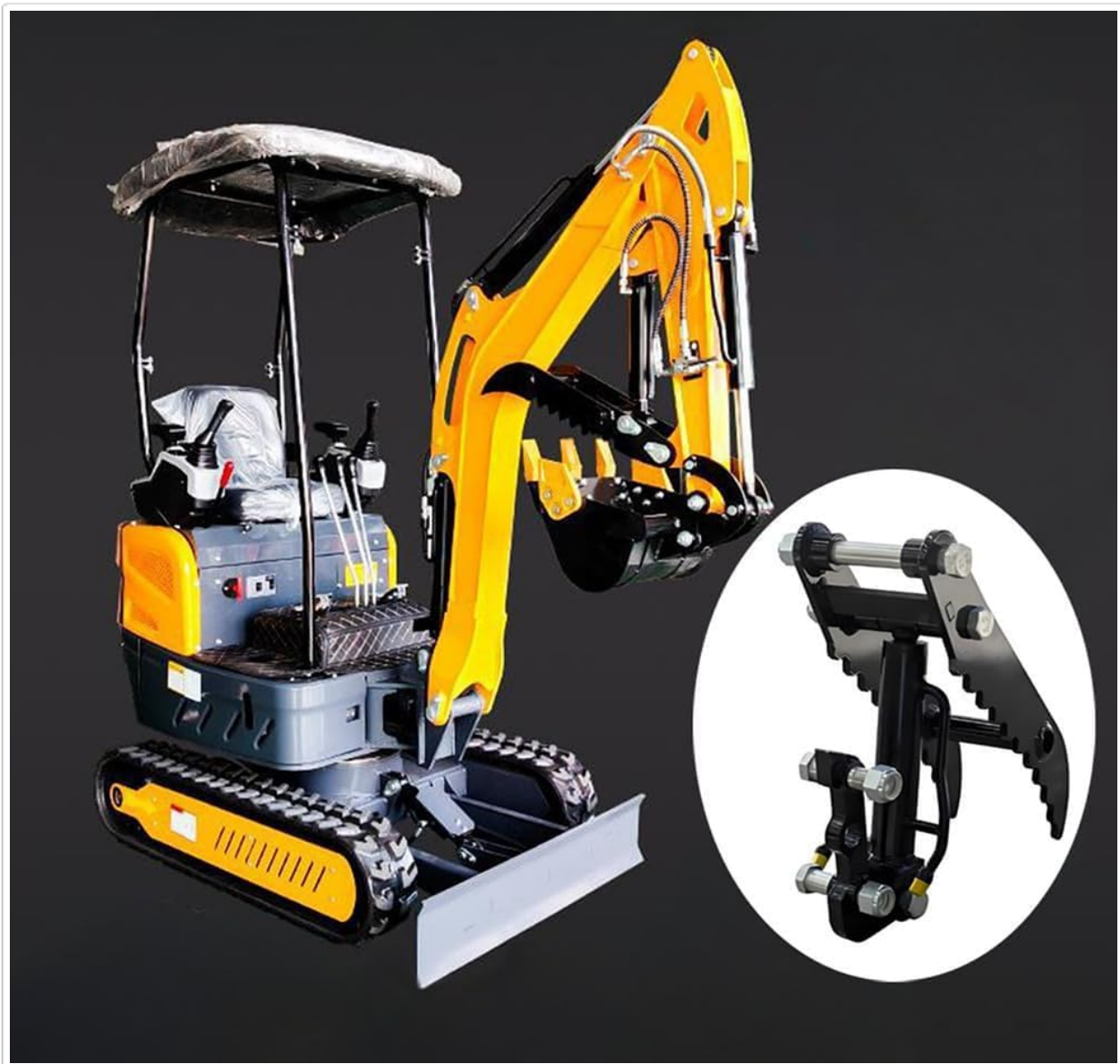
Image 4.1: An excavator with the hydraulic thumb clip installed, demonstrating its integration.
