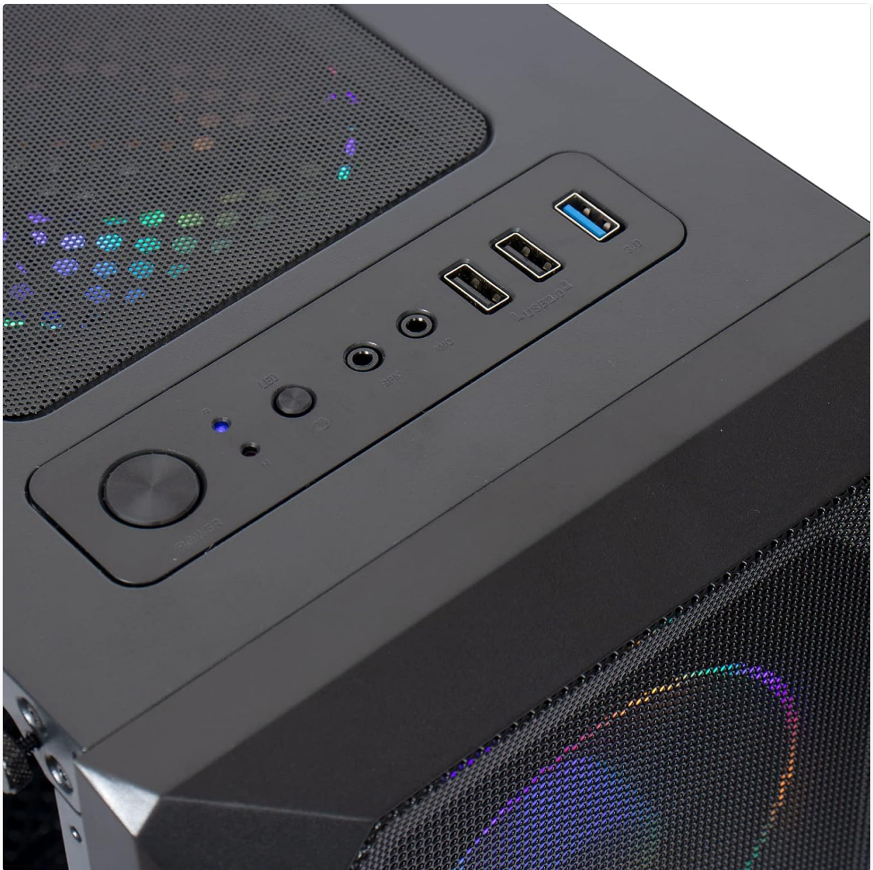
Figure 2.2: Top-mounted front I/O ports including USB and audio jacks.
