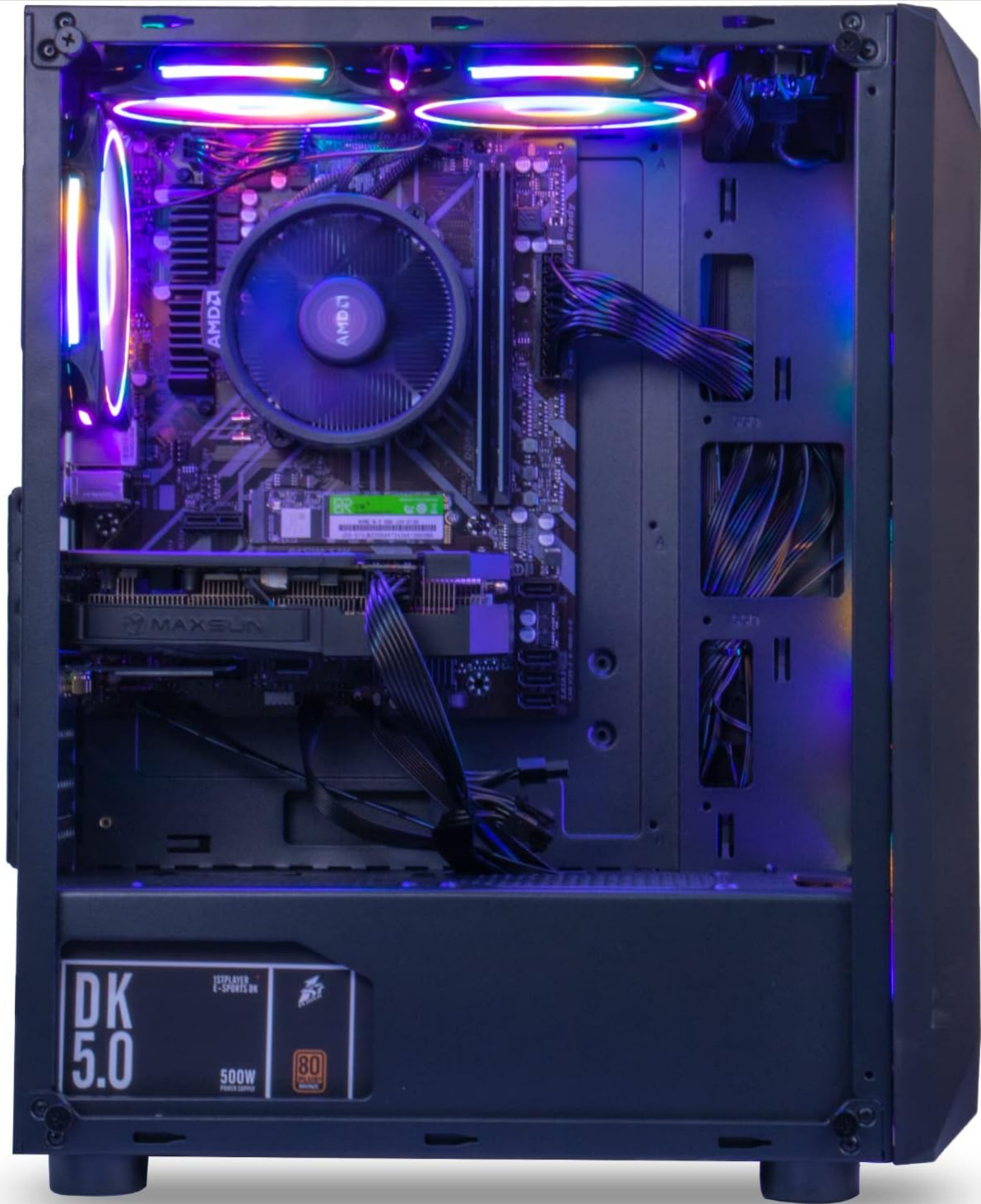
Figure 3.2: Internal layout of the MXZ Gaming PC, showcasing the motherboard, GPU, and power supply.
