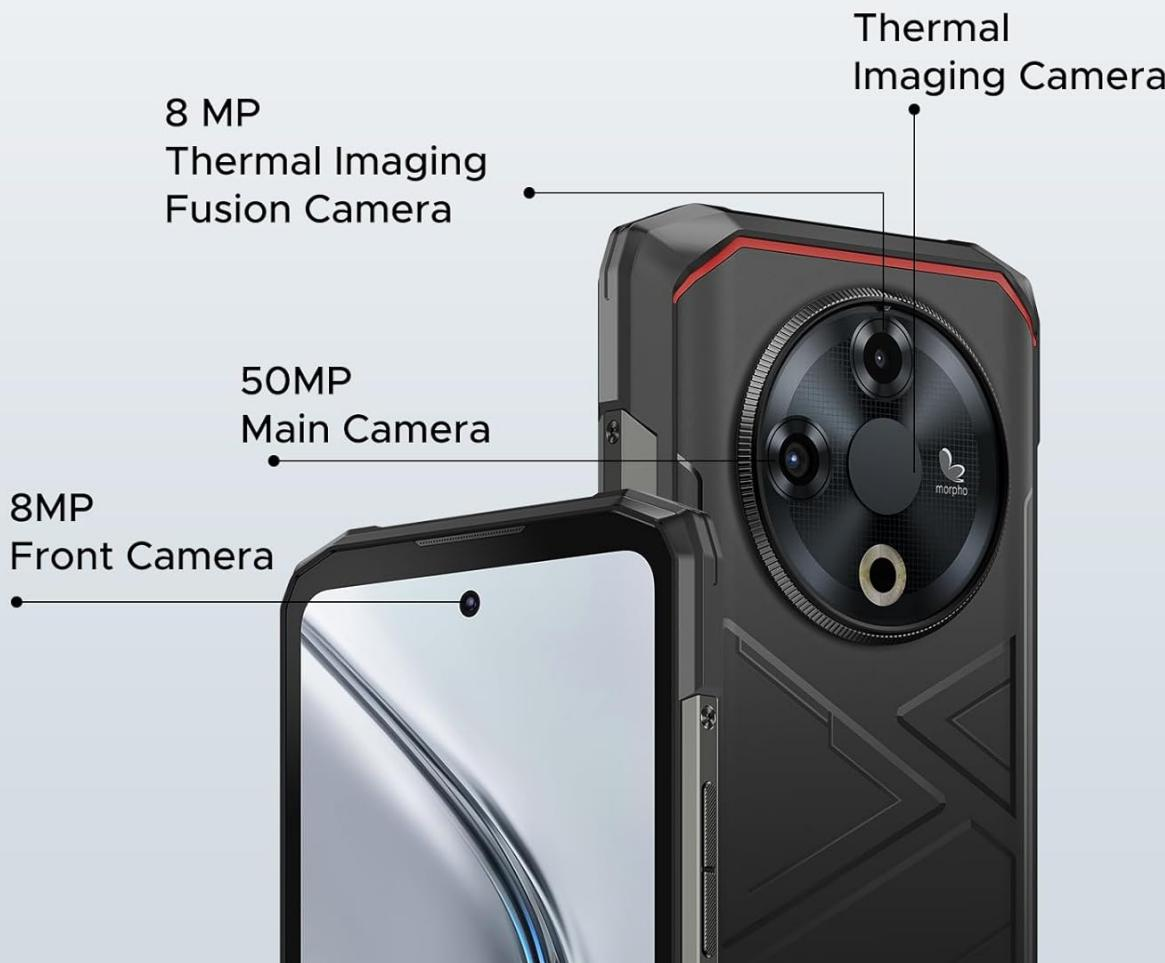
**Advanced Camera System:** The Fire 6 includes a 50MP AI main camera, an 8MP front camera, and an 8MP fusion lens. It supports dual-light fusion technology for improved low-light performance and features like HDR, portrait, and panorama modes.
