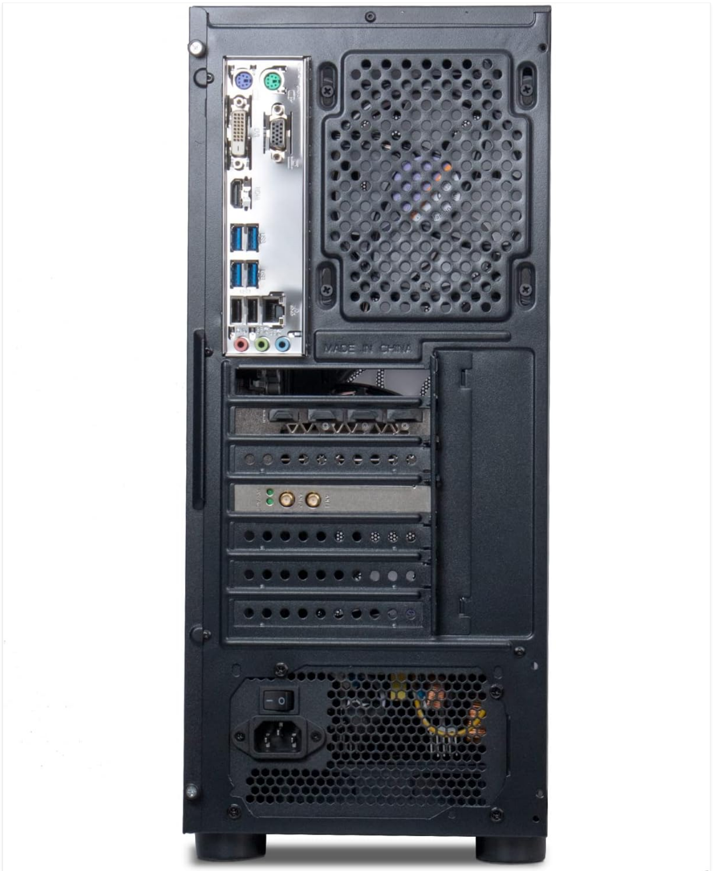
Figure 4.4: Rear view of the MXZ Gaming PC, displaying the motherboard I/O shield with USB ports, audio jacks, Ethernet port, and the dedicated graphics card output ports (HDMI, DisplayPort).
