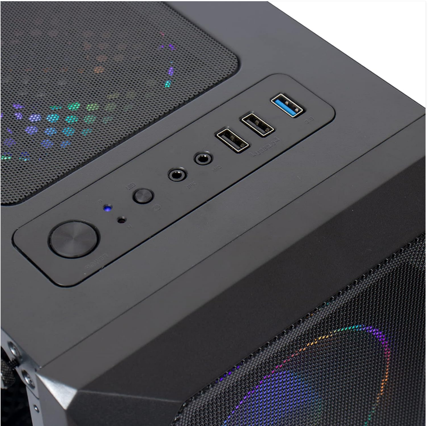
Figure 4.3: Close-up of the top panel, featuring power button, reset button, USB 2.0 ports, USB 3.0 port, and audio jacks for convenient access.
