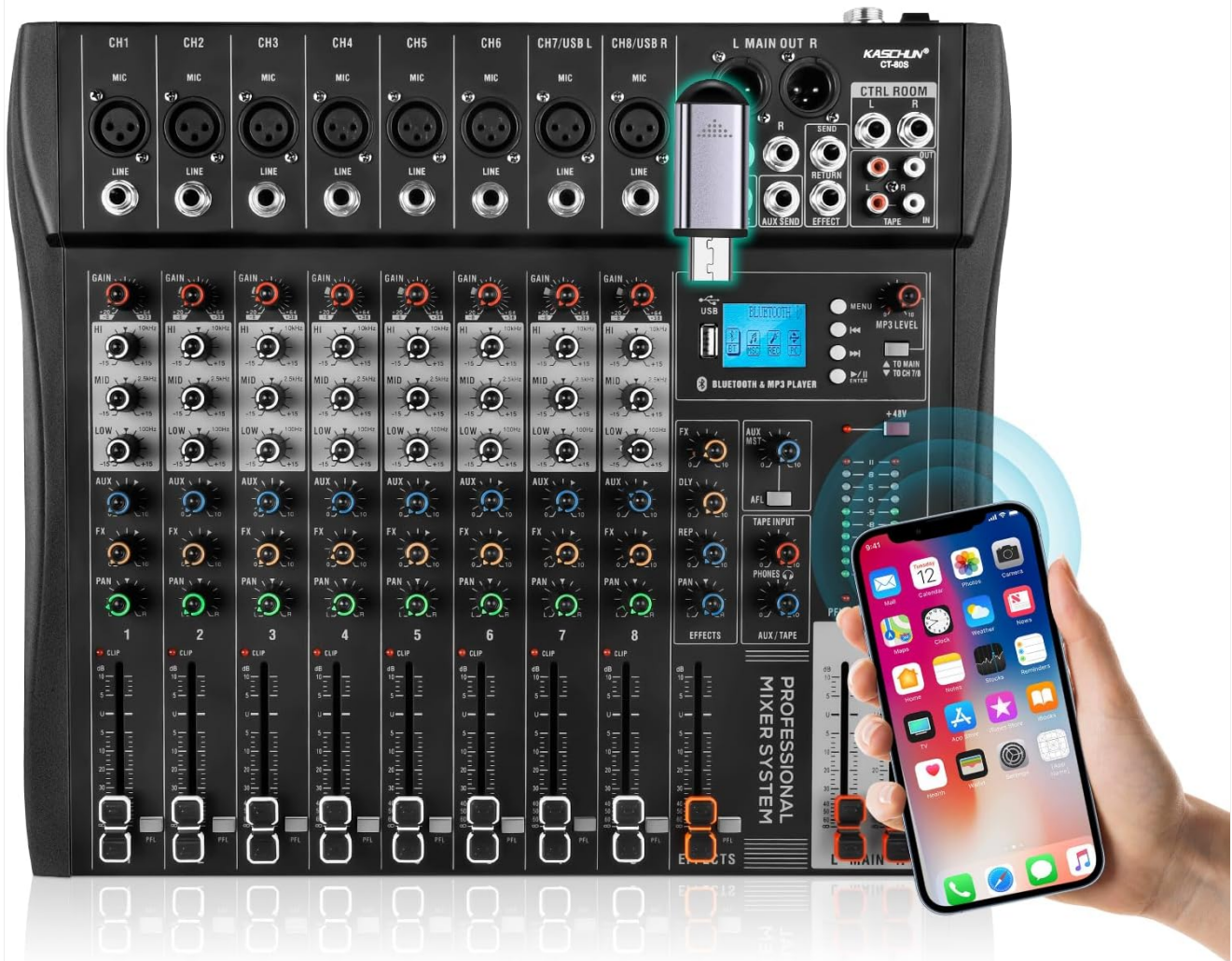
Figure 5.1: Illustration of Bluetooth wireless connection to the CT120S mixer from a mobile device.
