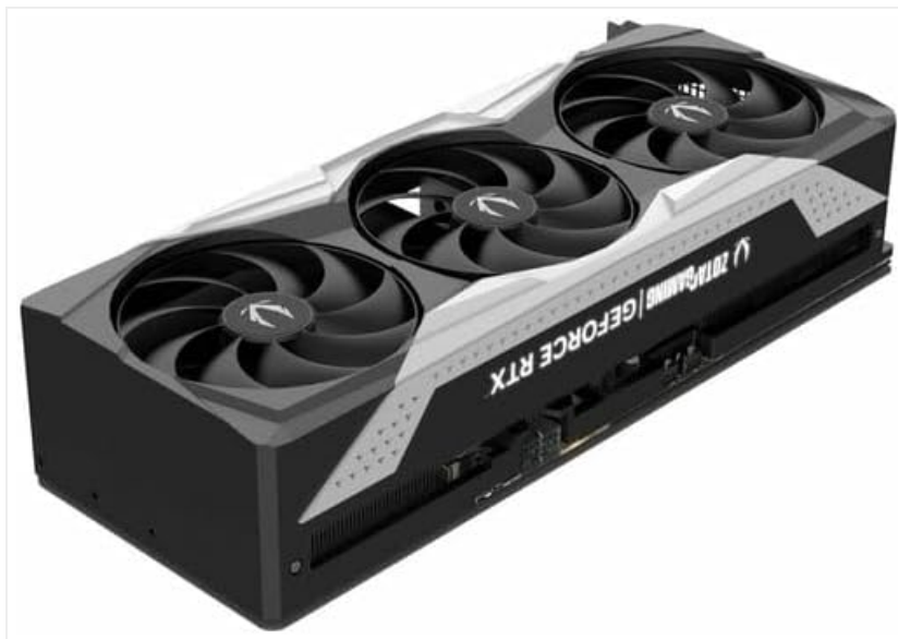
Image 6.1: Angled view of the graphics card, highlighting its robust cooling solution.
