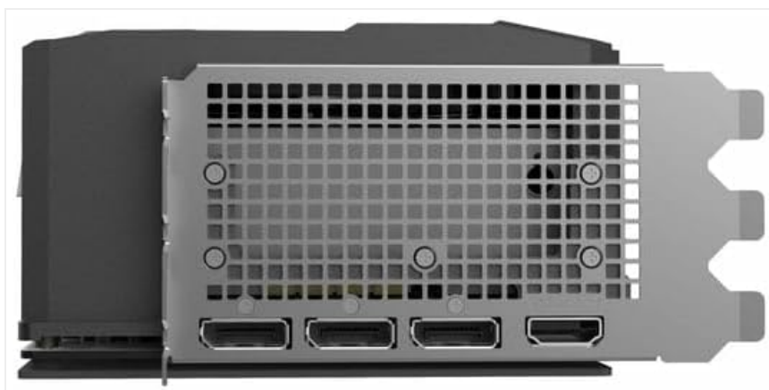
Image 4.2: Rear view of the graphics card, showing three DisplayPort outputs and one HDMI output.
