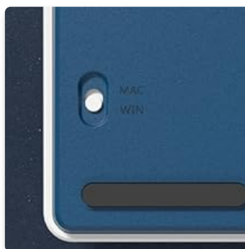
Figure 5: Close-up of the Mac/Win compatibility switch on the keyboard's underside.
