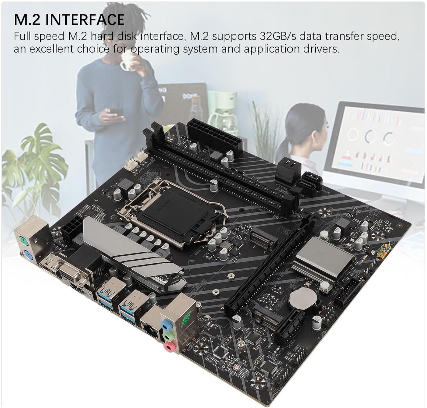
Image 3.3: The M.2 interface, designed for high-speed NVMe SSDs.
