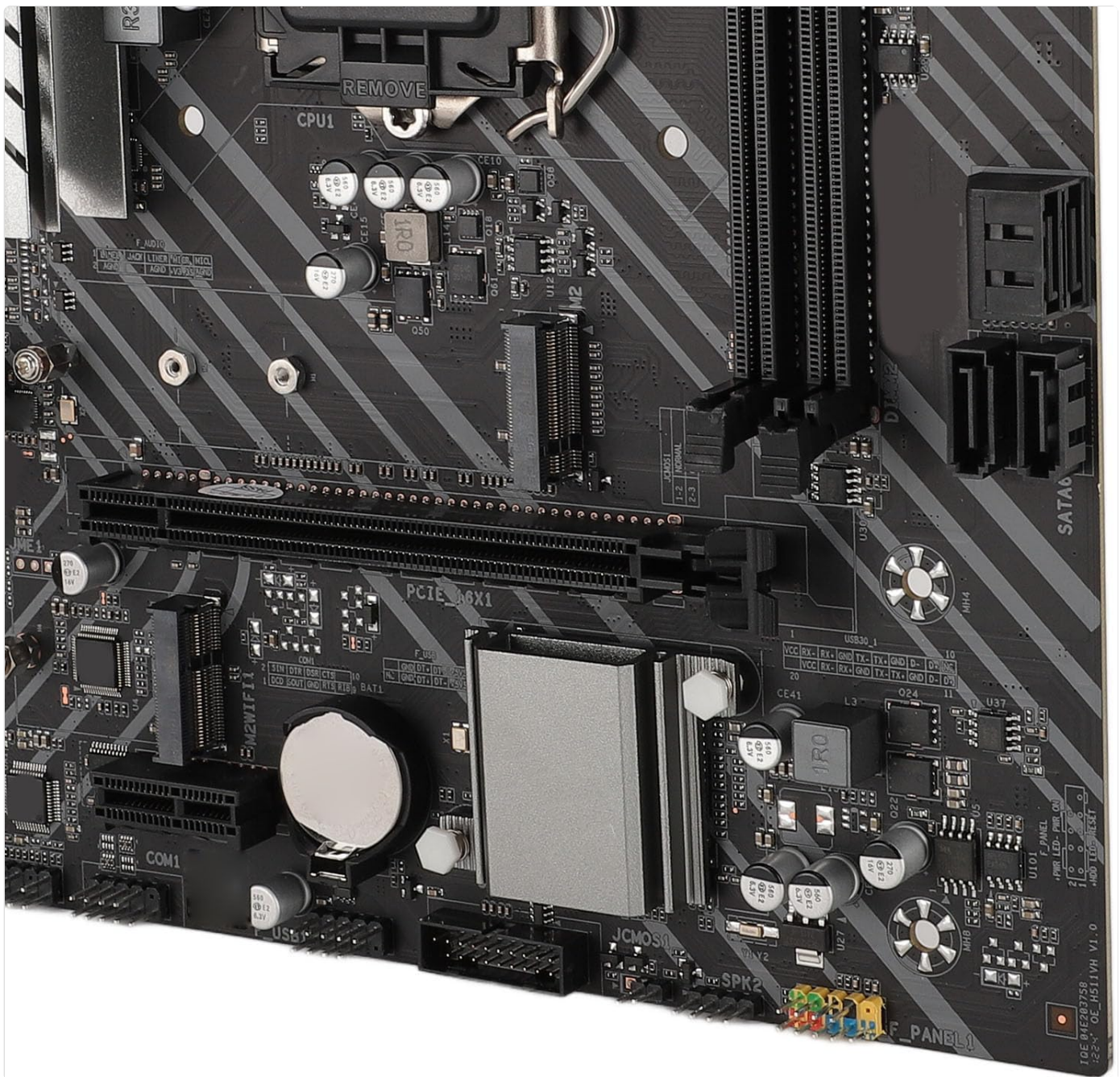
Image 3.4: Close-up of the M.2 slot and surrounding expansion slots and headers.
