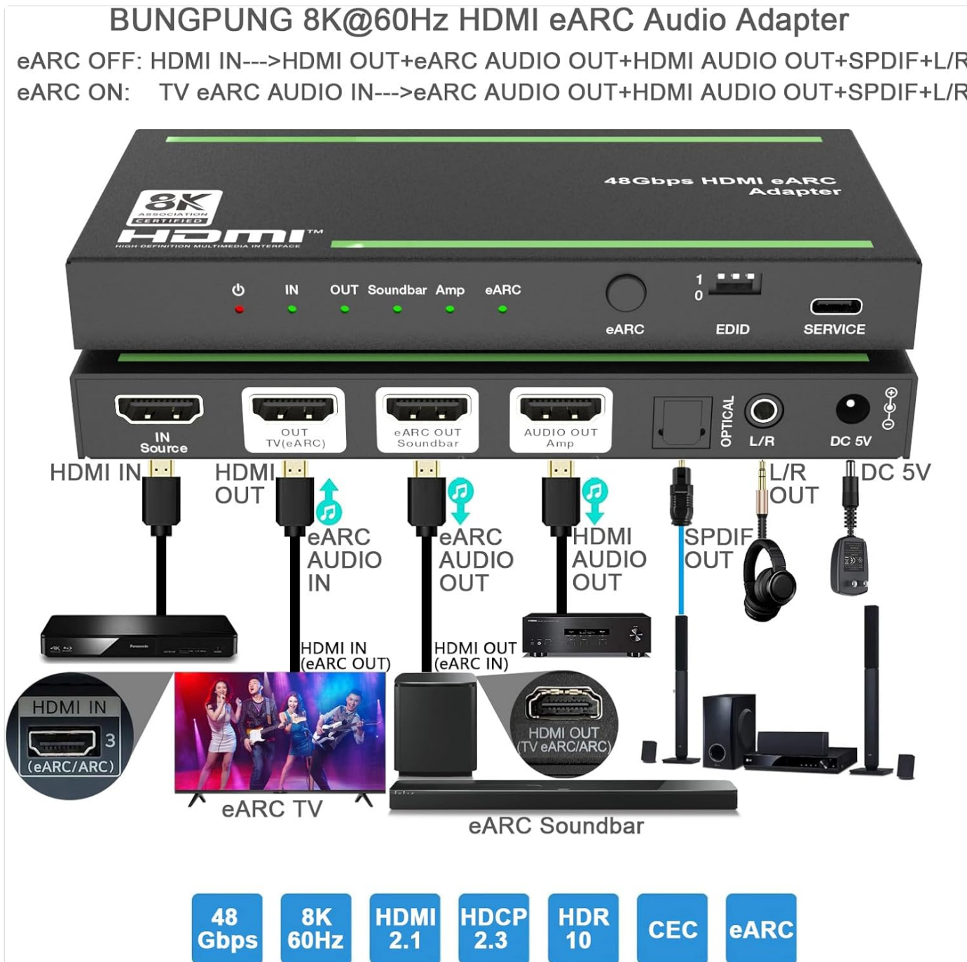
Figure 6: Connection Diagram for eARC ON Mode
