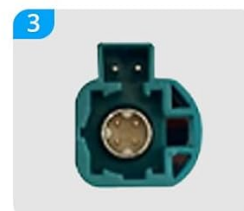
6-pin LVDS Connector at the Rear of OEM Display
