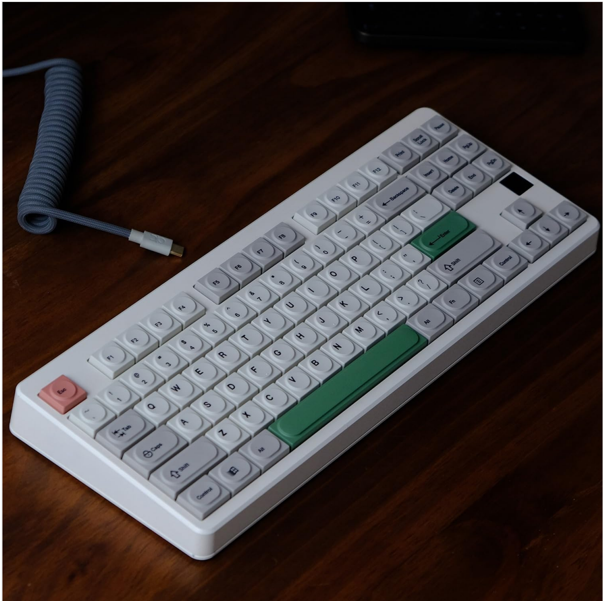
Image 1.1: LPkeybd 9009 Low Profile Keycaps installed on a mechanical keyboard, showcasing the retro color scheme and low profile.
