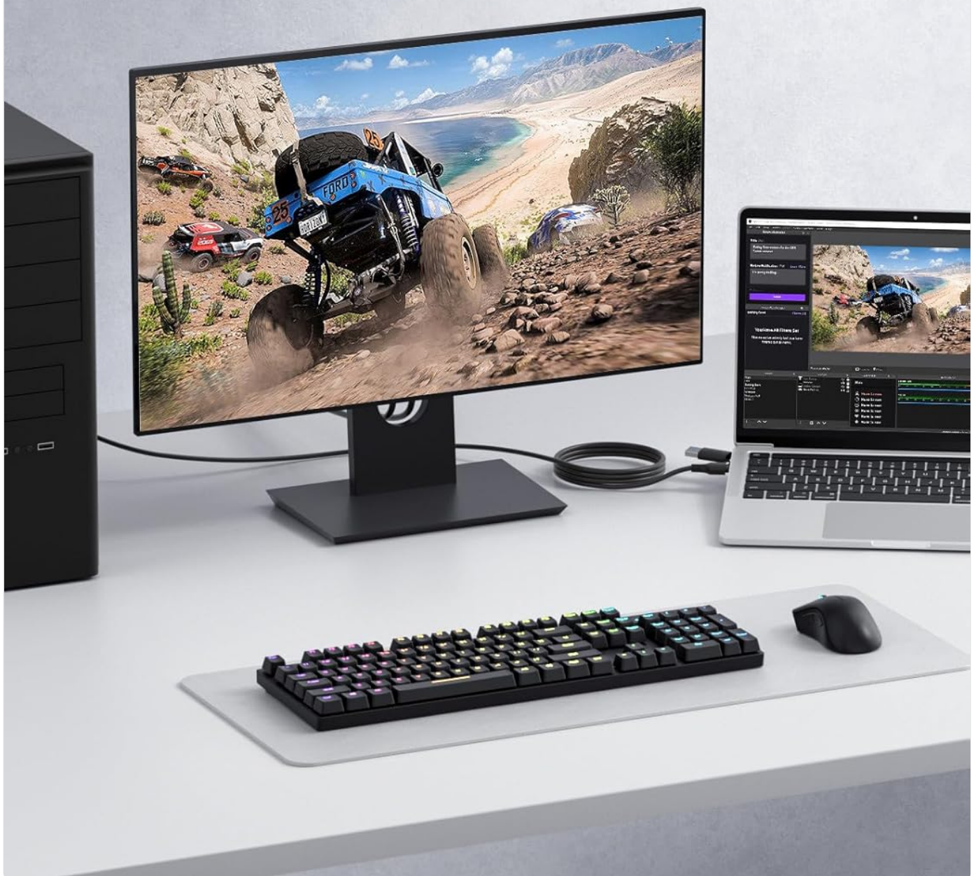
Figure 6: Configuration for recording or live streaming computer games using the capture card.
