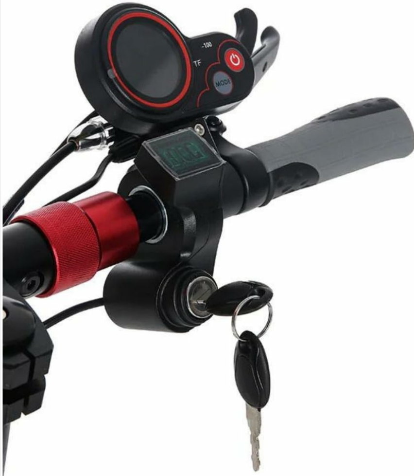
Image 3.2: The TF-100 throttle unit mounted on an electric scooter's handlebars, showing its position relative to other controls.
