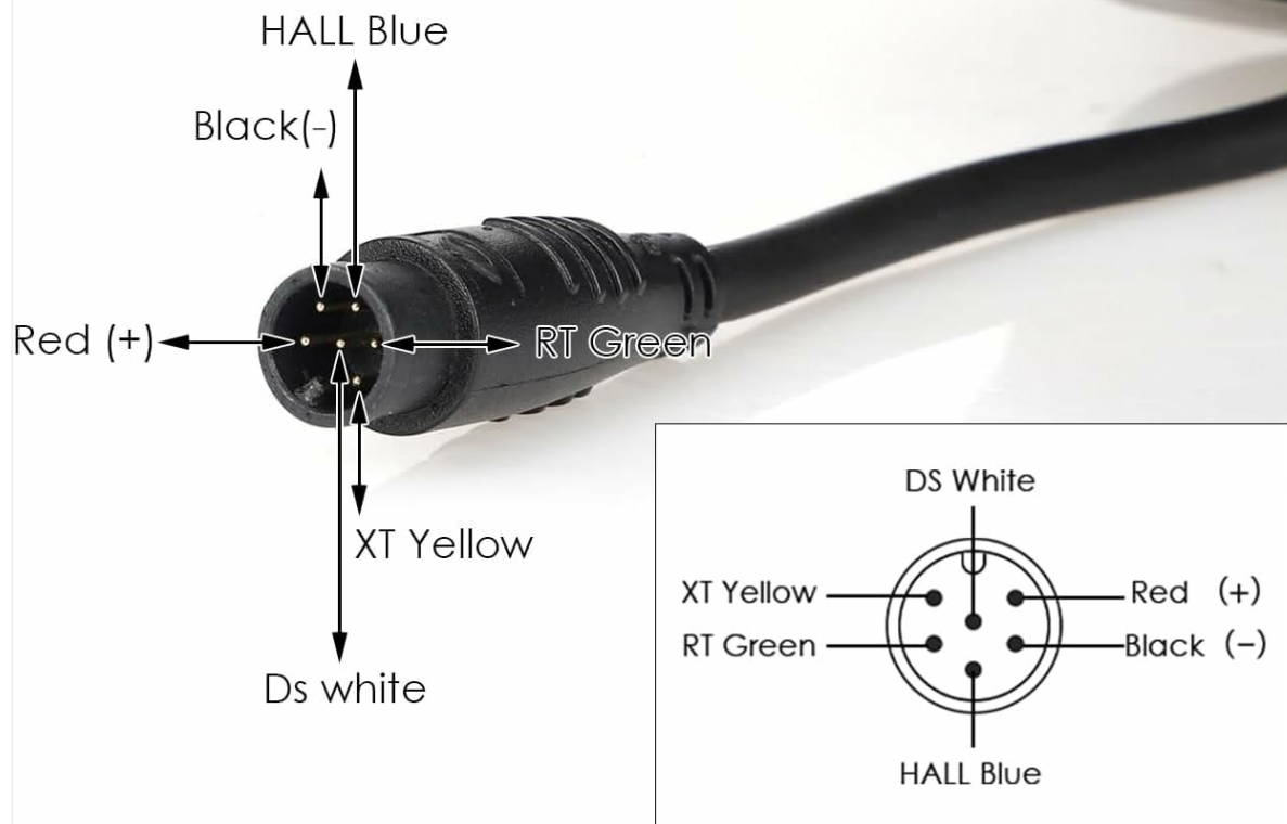
Image 3.1: Detailed 6-pin wiring diagram. Pin assignments are: Red (+) for positive power, Black (-) for negative power, HALL Blue, RT Green, XT Yellow, and DS White for signal and data lines.
