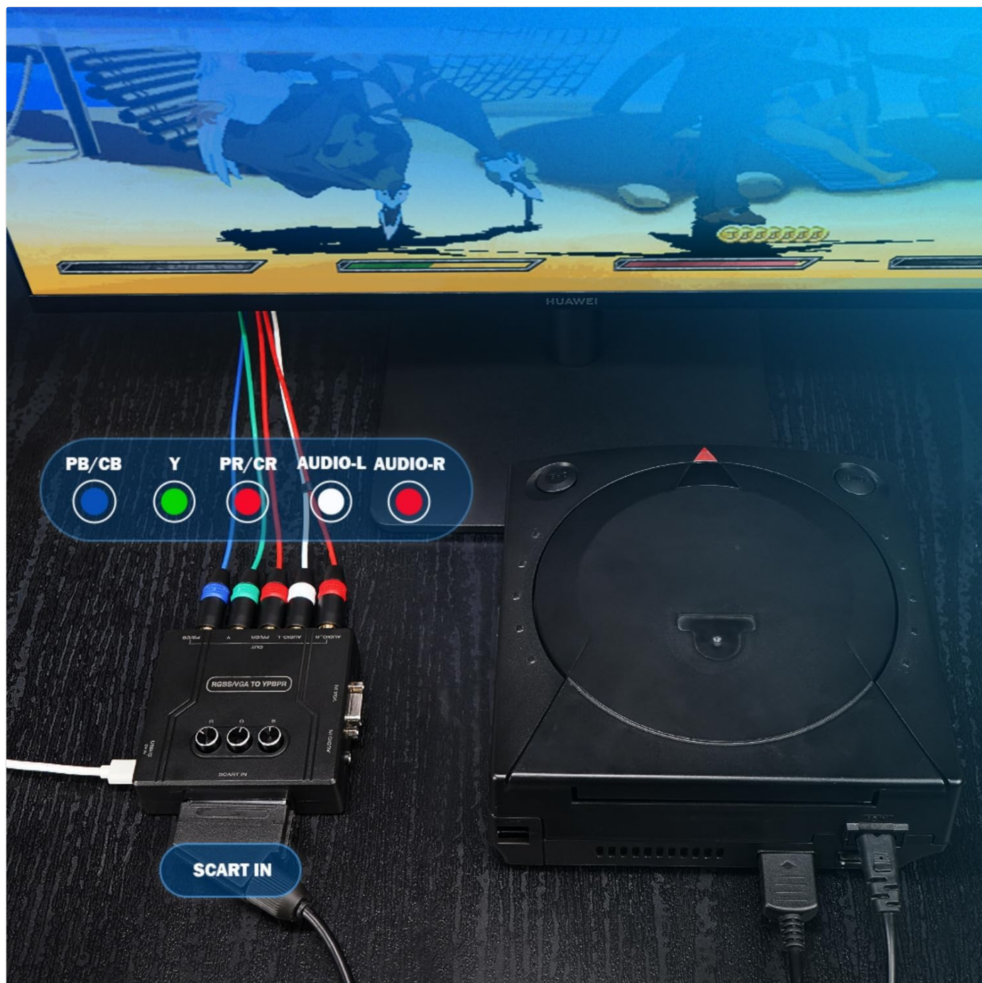
Figure 6: Example setup with a Dreamcast console connected to the converter via SCART, and the converter outputting component video to a monitor.
