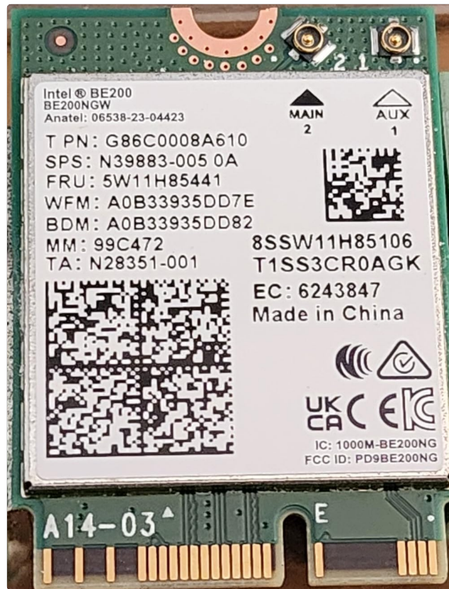
Figure 1.1: Front view of the Intel Wi-Fi 7 BE200 network card, showing the Intel branding, model number, and various regulatory markings.
