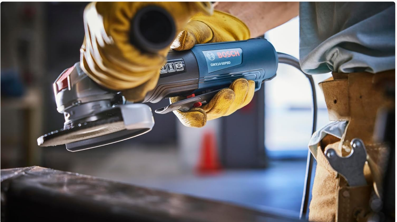
Image: A hand attaching the anti-vibration side handle to the BOSCH GWX14-50PBD Angle Grinder.
