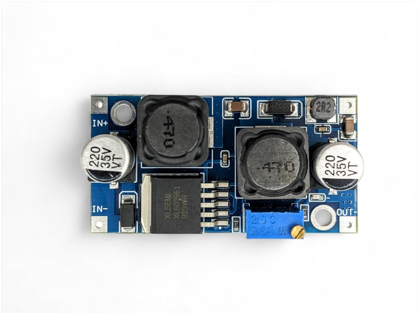
Figure 1: Angled view of the XL6009 module, highlighting the IN+ (Input Positive), IN- (Input Negative), OUT+ (Output Positive), and OUT- (Output Negative) terminals.
