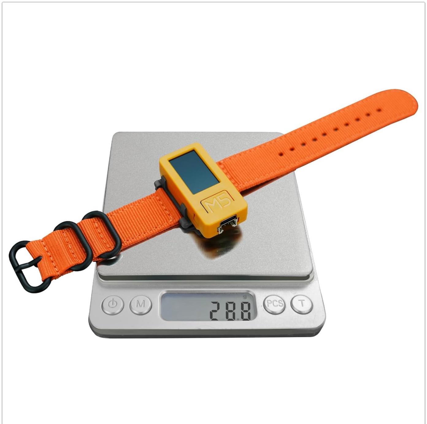
Figure 7.3: M5StickC PLUS2 Weight. The device, attached to its watch strap, is shown on a digital scale displaying a weight of 28.8 grams.
