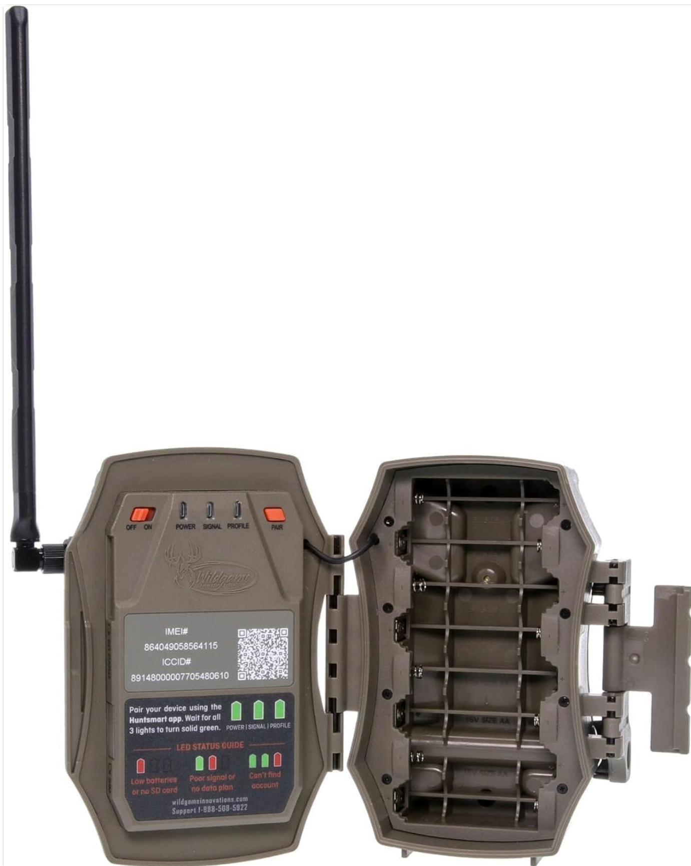
Figure 3: Internal view of the camera, highlighting the battery slots and the QR code for app setup.
