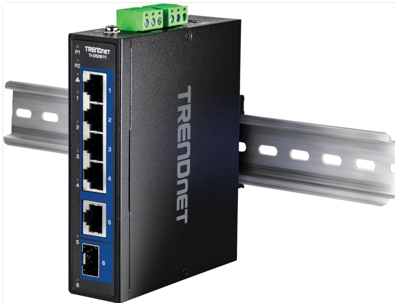
Figure 5: Power and alarm terminal blocks on the rear of the switch.
