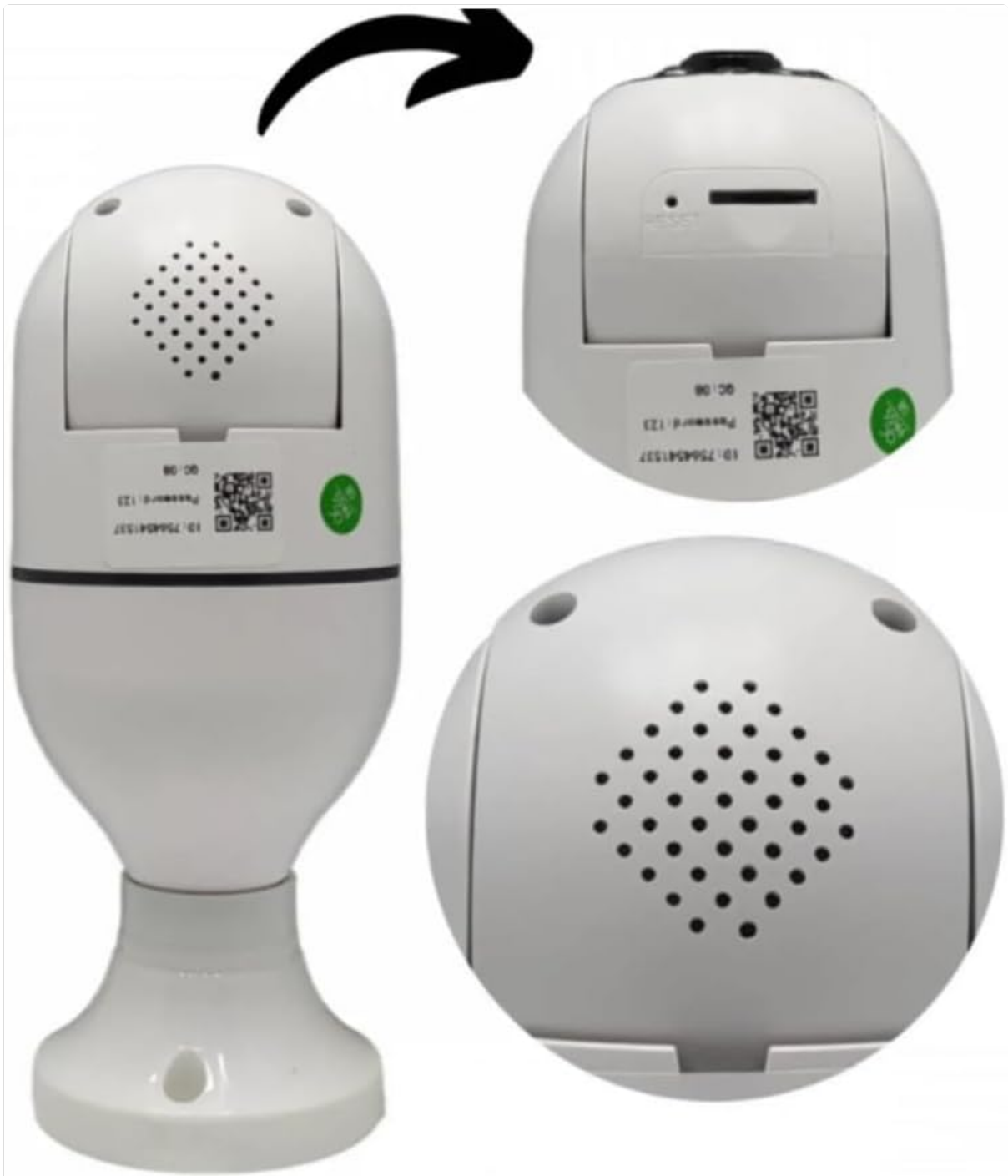
Image 4.2: Rear view of the camera, highlighting the reset button and SD card slot.
