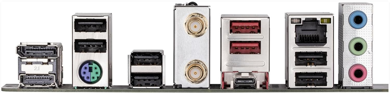
Figure 4: The rear I/O panel provides various ports including USB, Ethernet, Wi-Fi antenna connectors, and audio jacks.
