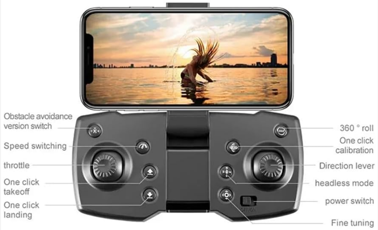
Image 3.2: Detailed diagram of the remote control, indicating functions such as speed switching, one-click takeoff/landing, throttle, direction lever, headless mode, power switch, and fine tuning.
