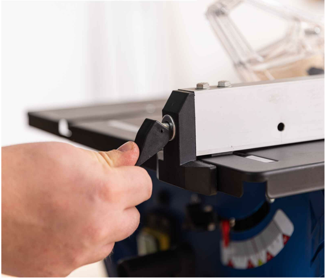
Figure 4.3: The rip fence, clamped on both sides, with an integrated scale for particularly precise longitudinal cuts.
