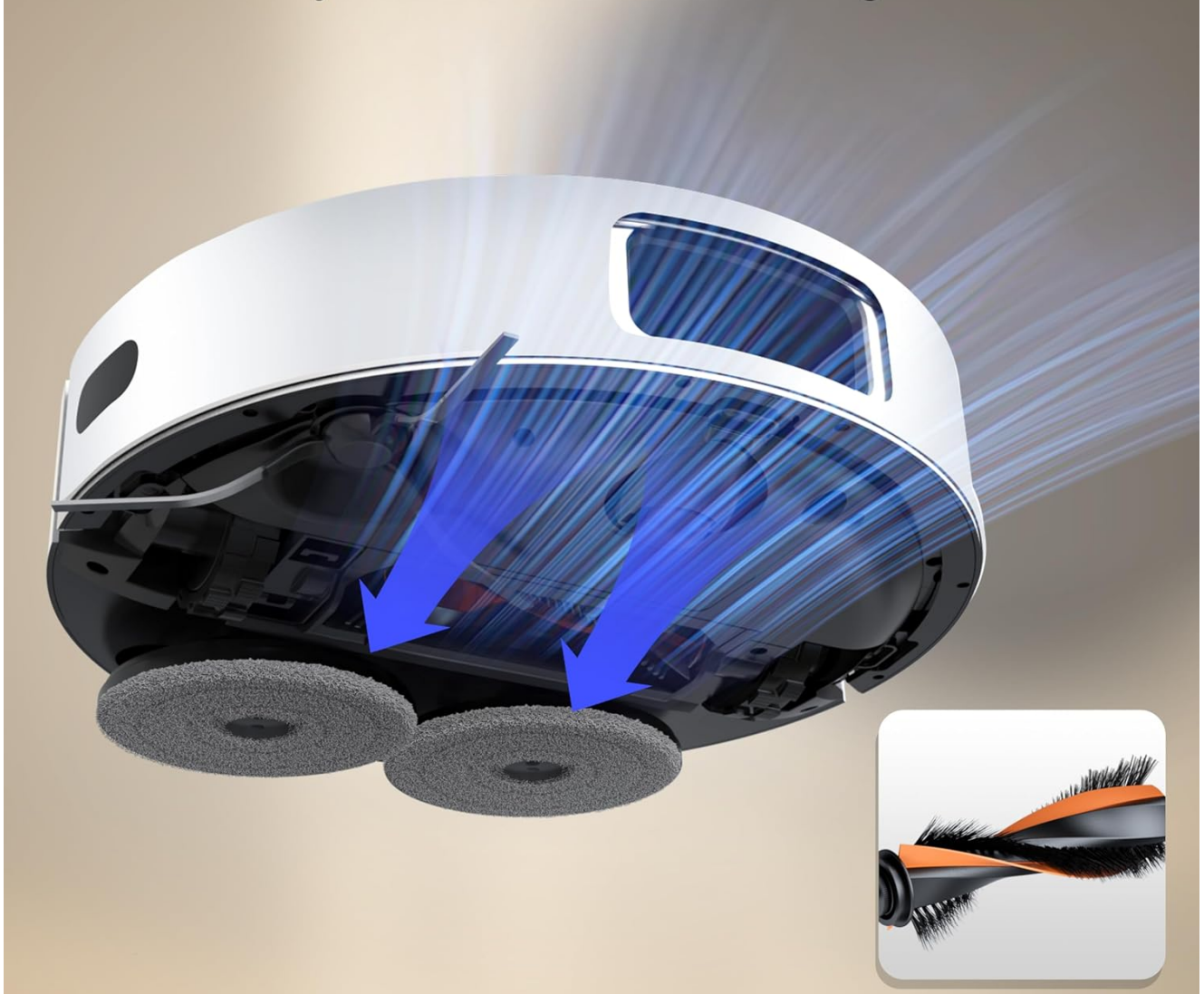
Figure 5.2: Close-up view of the robot's anti-tangle design roller brush, which uses cyclone air flow to prevent hair from wrapping around it.
