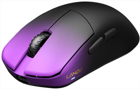
Figure 4: A front-side perspective of the Lamzu Maya X mouse, displaying its symmetrical shape and the USB-C charging/wired connection port at the front.
