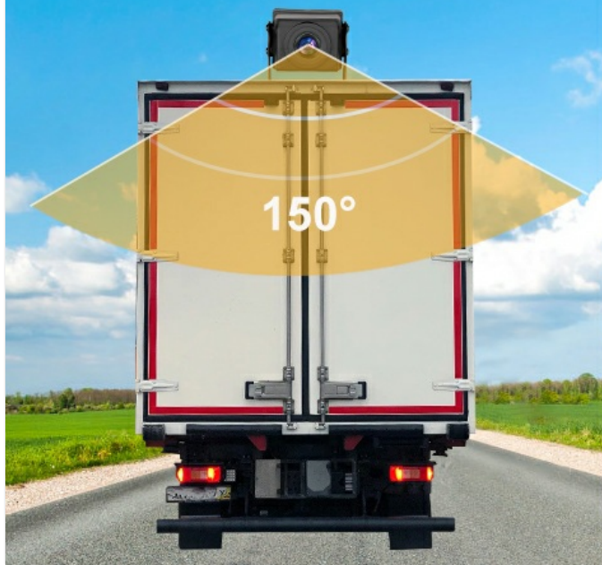
Image: Visual demonstration of the 150-degree wide-angle view from the camera and the clarity of the 1080P HD resolution on the monitor.
