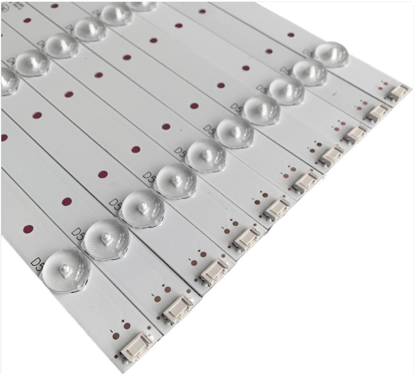
Image 3: A closer look at the LED lenses on the backlight bar.
