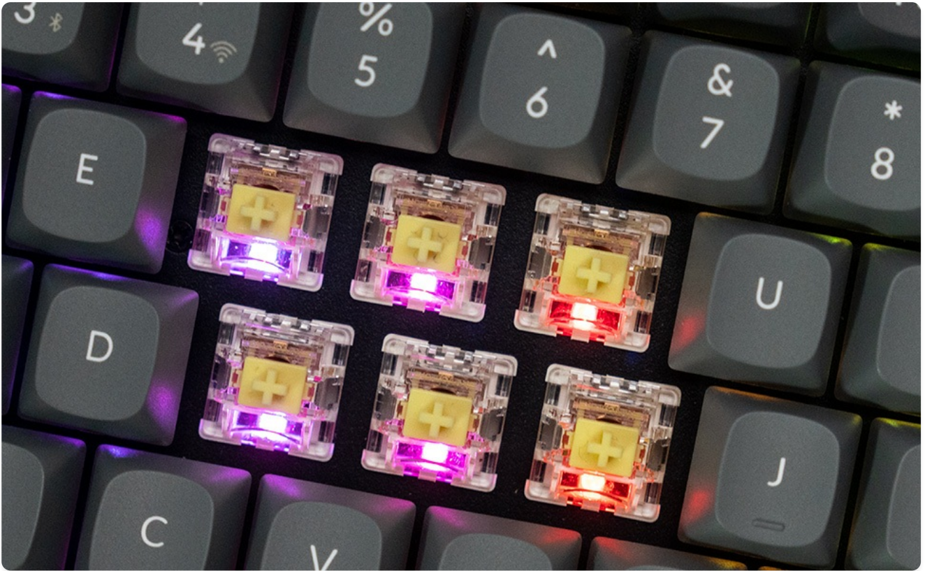
A close-up of the mechanical switches, illustrating their design and the RGB lighting capabilities.
