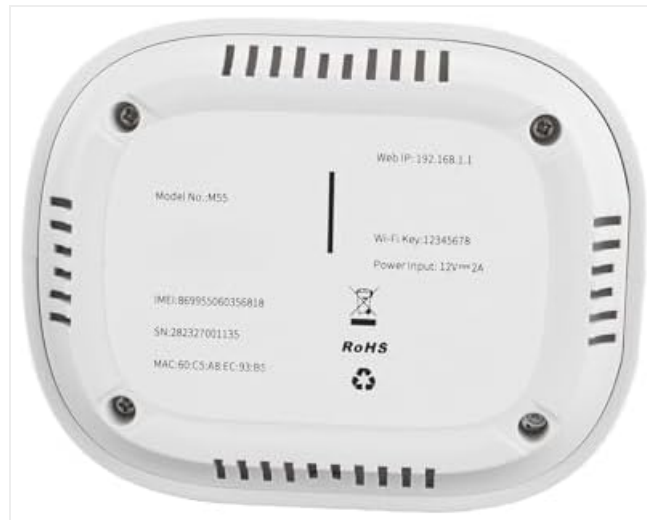
Image: The bottom surface of the Dpofirs 5G Router, displaying important information such as Model No.: M55, Web IP: 192.168.1.1, Wi-Fi Key: 12345678, and Power Input: 12V=2A. This information is crucial for initial setup and access.
