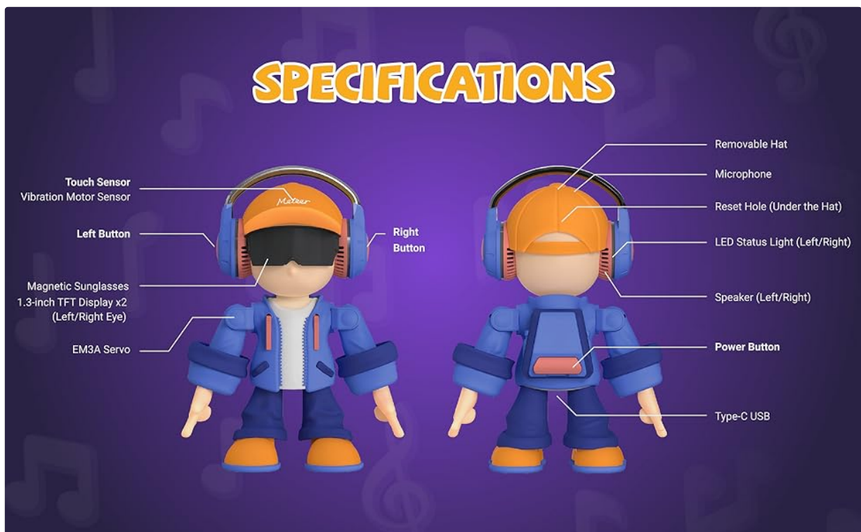
Image 4.1: Diagram illustrating the Meter robot's physical controls and components, including touch sensor, buttons, and display.
