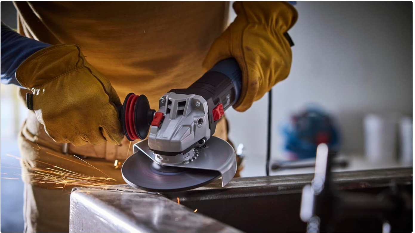
Figure 5: Angle grinder in use for metal cutting.
