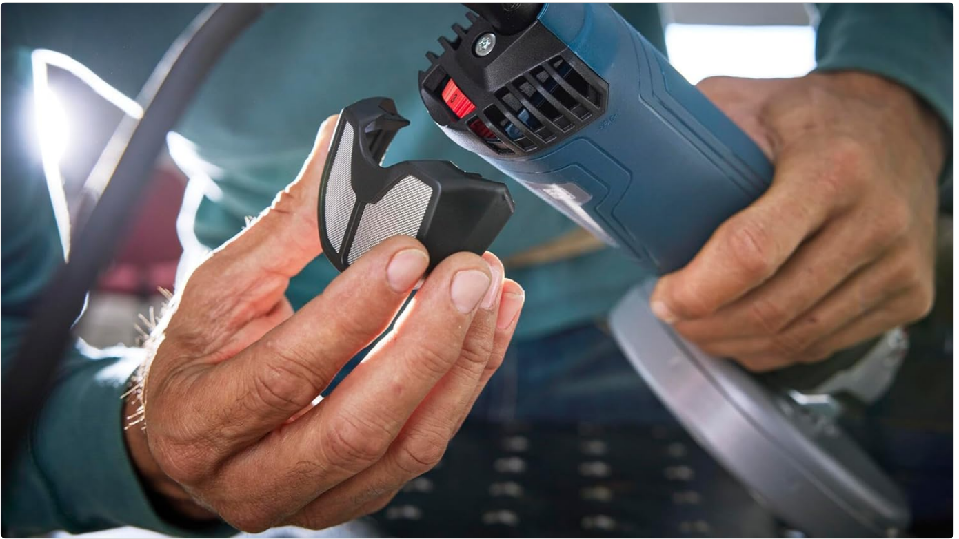
Figure 6: Removing and cleaning the air filter.
