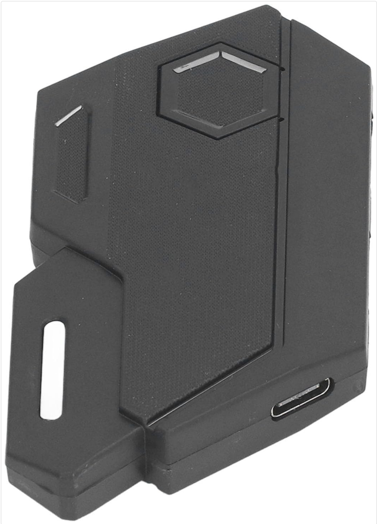
Figure 3.7: Close-up side view of the converter, highlighting the Type-C input port used for power supply and charging the connected mobile device.
