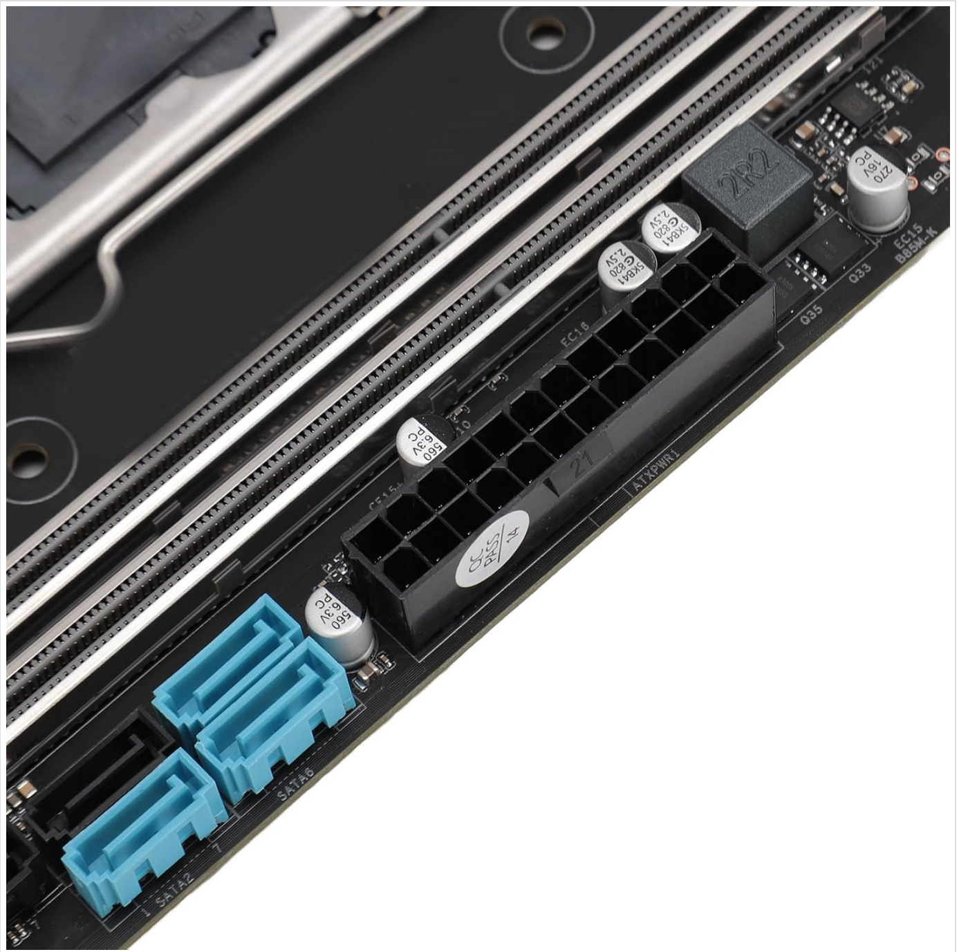
Image 7: Close-up of 24-Pin ATX Power Connector and SATA Ports. This image details the main power input for the motherboard and additional SATA ports.
