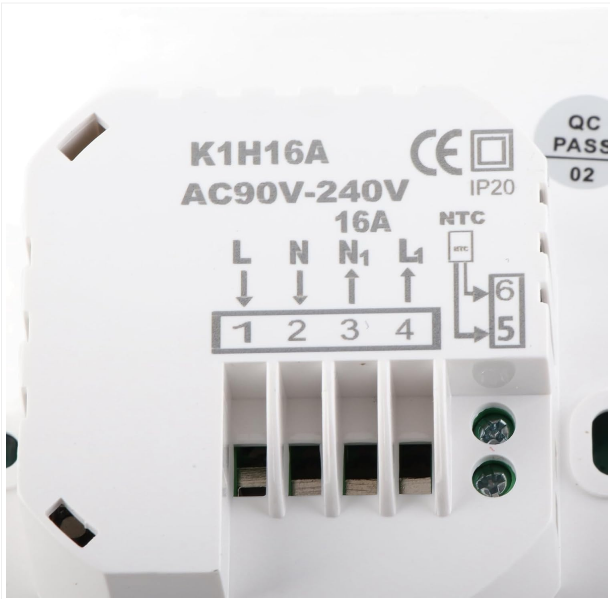
Image: Detailed view of the thermostat's rear, illustrating the wiring terminals (1-6) and the corresponding labels for Live, Neutral, Load, and NTC sensor connections. The model number K1H16A and voltage range AC90V-240V 16A are visible.
