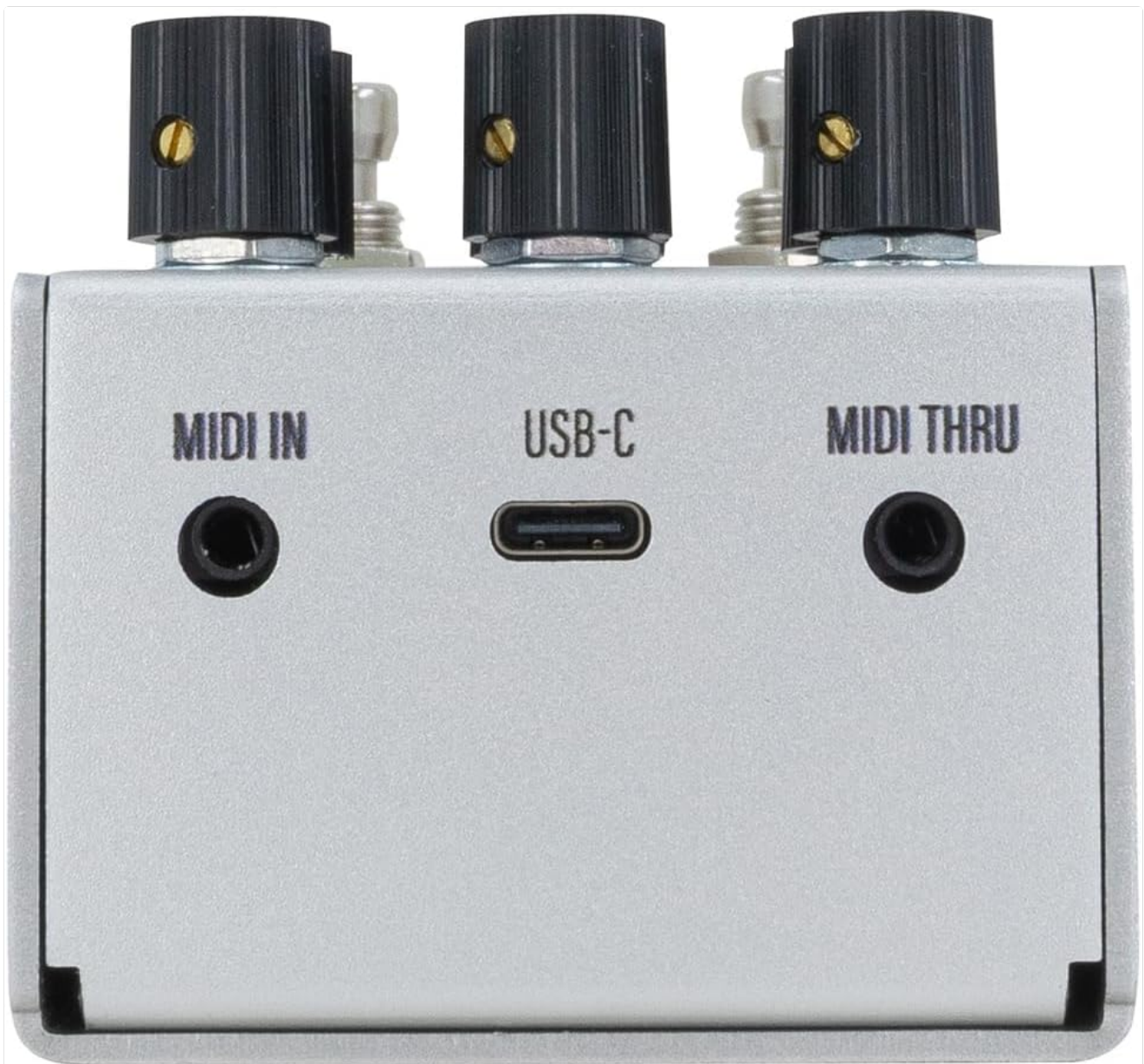
Figure 4: Rear view of the D1 MKII pedal, showing MIDI In, USB-C, and MIDI Thru ports.
