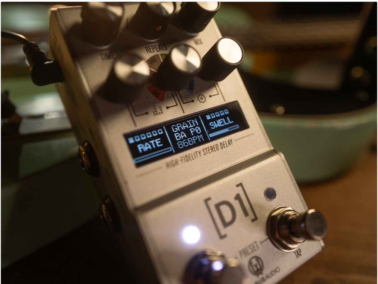
Figure 6: OLED display showing parameters for the Grain delay algorithm.
