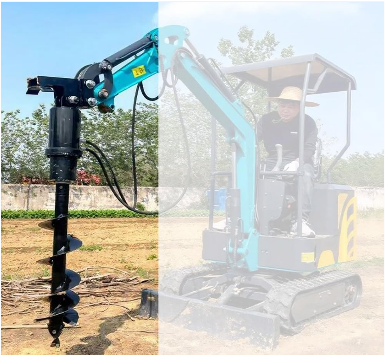
Image 1.1: Mini excavator utilizing the auger attachment for drilling.
